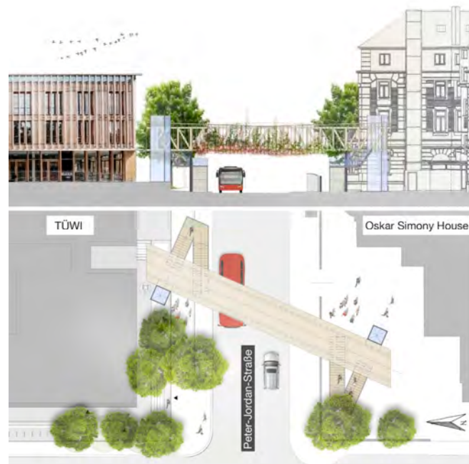
Figure 15. Layout and side view of the dynamic rotated version put in context with the adjacent buildings and pedestrian flows, without scale. © designkollektiv GmbH.
