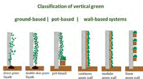
Figure 7. Simplified classification of vertical greening systems (based on [33]).
